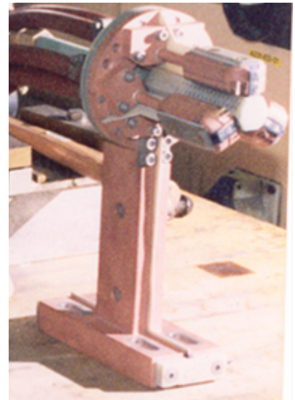
Induction coil for CVJ hardening with Fluxtrol concentrators
