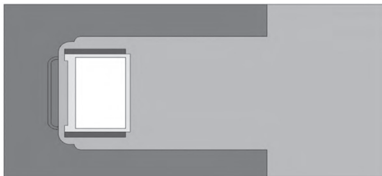
Fig. 16 Nonrotational inductor cross section used for simulation
