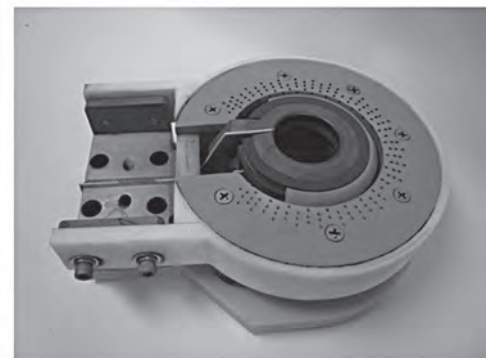
Fig. 27 Two-turn scan hardening coil with magnetic flux controllers used for axle scan hardening. Source: Ref 4
