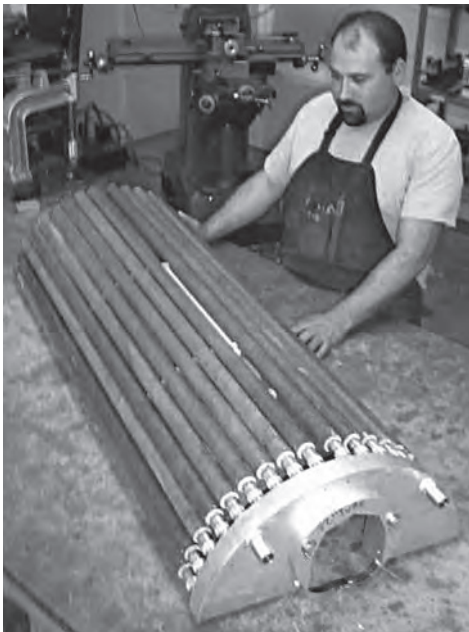
Fig. 23 Cluster impeder (multiple impederers assembled together) for large diameter pipe welding. Courtesy of Electronic Heating Equipment, Inc.
