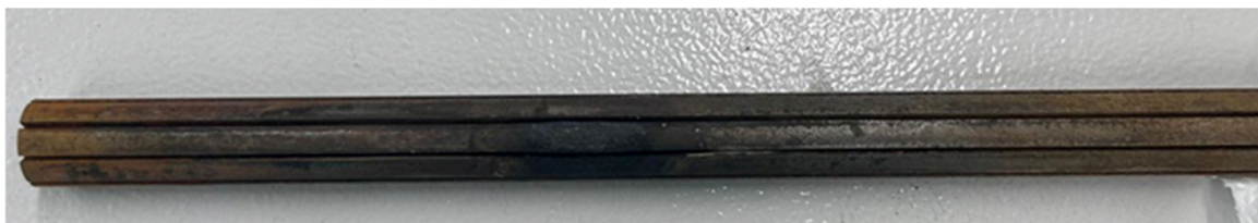
Figure 23. Thermally damaged Fluxtrol 50 impeder after a continuous test at a generator output of P_{el} = 13.5 kW.
