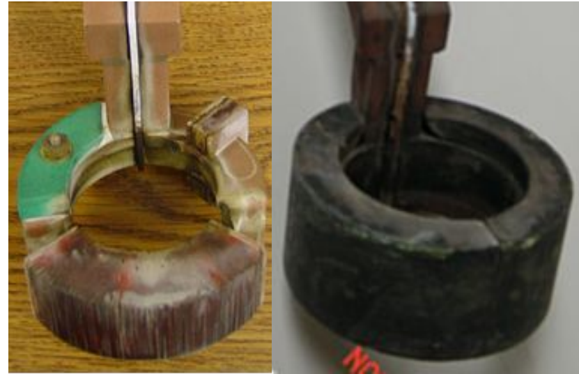
Original Coil (left) after 13,000 parts and Redesigned coil (right) after successfully heat treating over 180,000 parts
